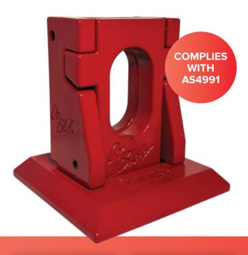
The OzBlok Road Plate Lifter system compromises of a receiver plate and a lifting tool. Once the receiver is flush welded at the centre of a steel trench plate, the lifting tool can be inserted into the receiver and locked into position before a hook is attached to the middle of the lifting tool. The flush welding reduces risk of tripping and allows for plates to be conveniently stacked.
